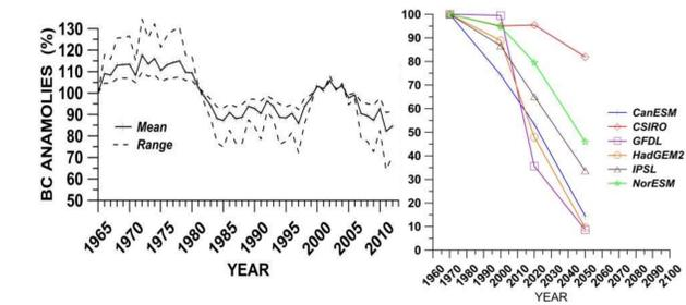
Figure 9. Left: Changes in foundation bearing capacity by 2013 using observational climate. Right: Changes in bearing capacity relative to 1970s using climate input from the six experiments
