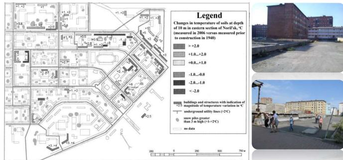
Figure 1. Left: Changes in permafrost temperature prior to construction and in 2006, for the eastern part of Norilsk. Right: Recently demolished buildings in Norilsk (photo by D. Streletskiy, July 2013)
